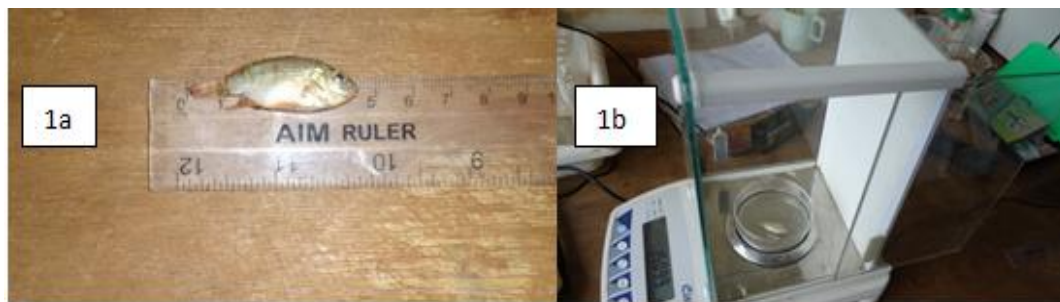
1. Measurement of growth parameters (a) length(cm) by a ruler and (b) weight(g) by a Citizen scale CY204, Poland, precision:0.0000 g
