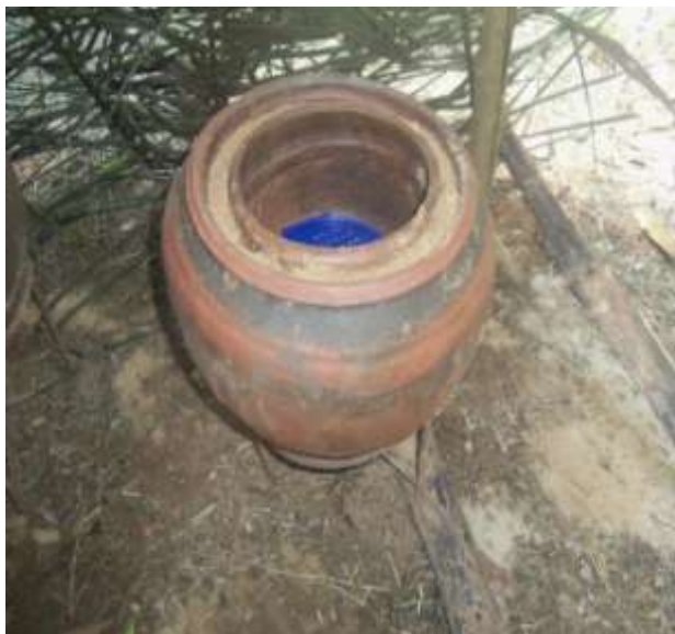
Figure 1: The Pot-in-Pot Evaporative Coolant Structure (26°C)
