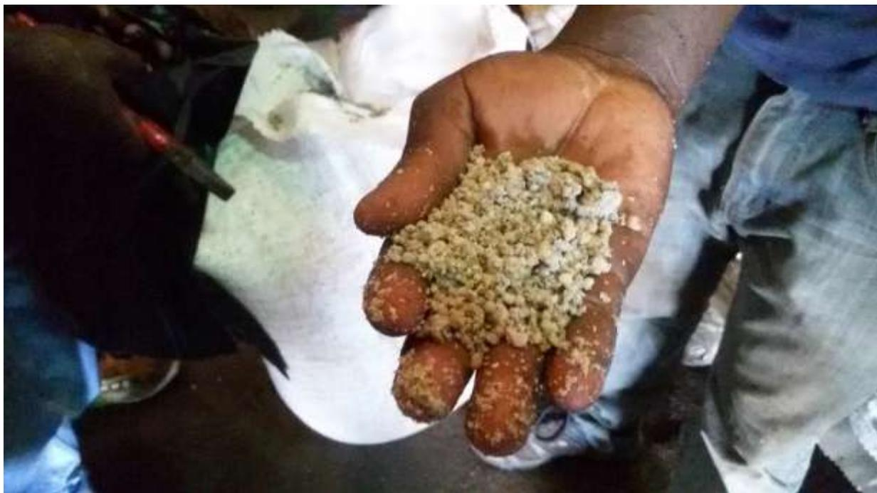
**Figure 3:** Sample of NPK fertilizer showing the moist condition of the fertilizer during storage
