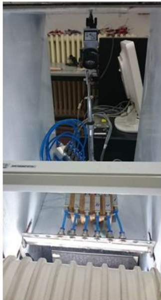
Figure 6. High-speed camera and pneumatic valves
