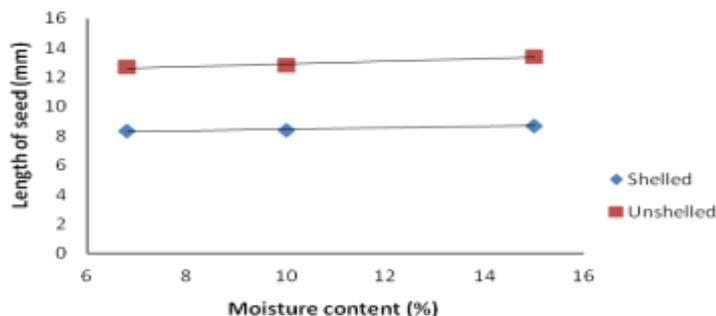
Fig 1 Effect of moisture content on length
