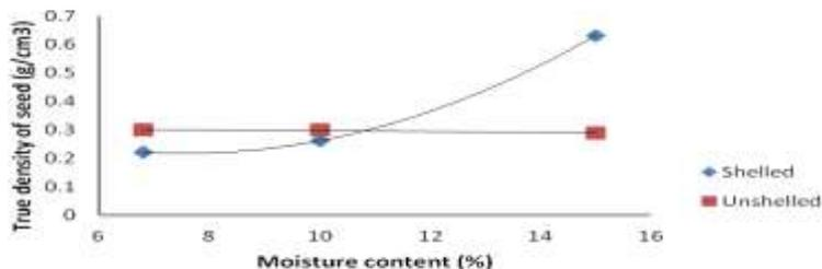
Fig 9: Effect of moisture content on true density
