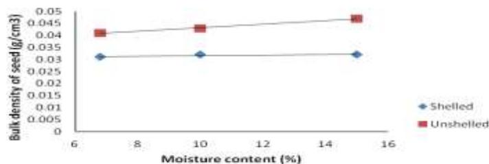
Fig 8: Effect of moisture content on bulk density
