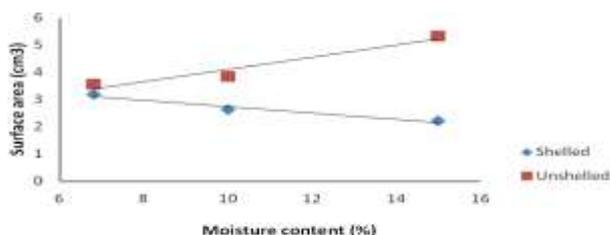
Fig 6: Effect of moisture content on surface area
