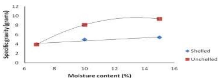
**Fig 15: Effect of moisture content on specific gravity**
