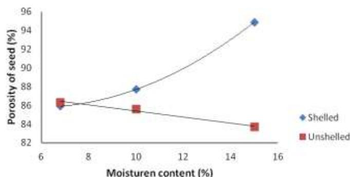
**Fig 10: Effect of moisture content on porosity**
