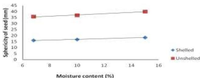
Fig 5 Effect of moisture content on sphericity
