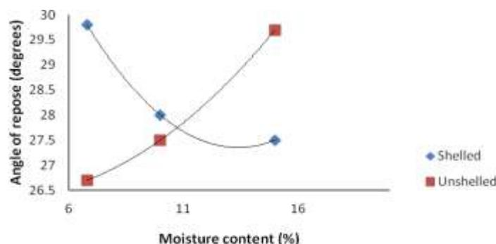
**Fig 11: Effect of moisture content on angle of repose**
