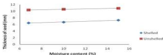
Fig 3 Effect of moisture content on thickness
