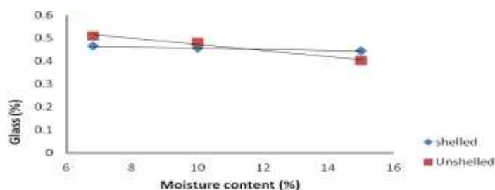
**Fig 12: Effect of moisture content on the static coefficient of friction of moringa seeds on a glass surface**
