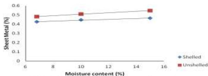
**Fig 13: Effect of moisture content on the static coefficient of friction of moringa seed on a metal surface**
