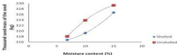
Fig 7: Effect of moisture content on thousand seed mass
