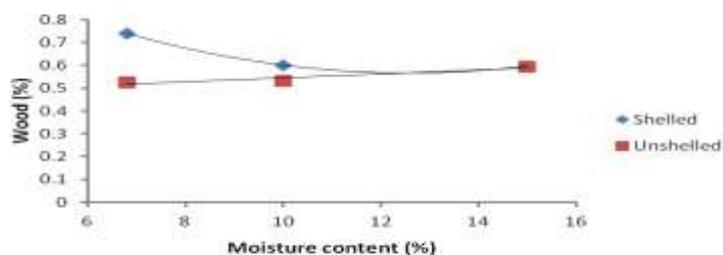
**Fig 14: Effect of moisture content on the static coefficient of friction of moringa seed on a wooden surface**
