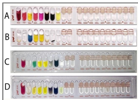
Figure 2: Biochemical reaction of API 20NE (A) Positive test, (B) Negative test, (C) Pseudomonas syringae pv. syringae and (D) Pseudomonas syringae .
