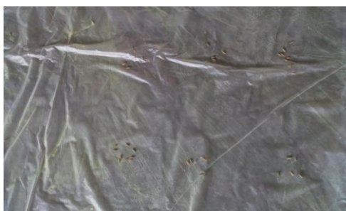
Plate 3.6 Hill dropping pattern of direct paddy drum seeder
