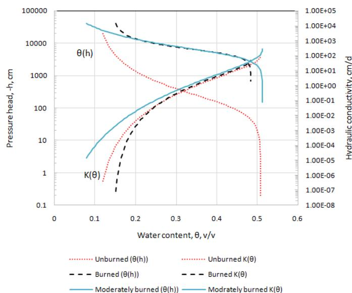
Fig. 1: Water retention  $h(\theta)$  and (transmission) hydraulic conductivity  $K(\theta)$  curves for the treatments
