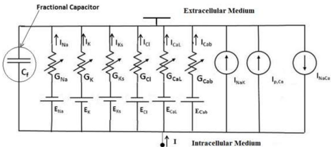
Figure 5: Electrical abstraction of the cardiac cell membrane.  $C_f$  is the fractional capacitor.  $G_{Na}$ ,  $G_K$ ,  $G_{Ks}$ ,  $G_{Cl}$ ,  $G_{CaL}$ , and  $G_{Cab}$  are conductances of  $Na^+$  ions,  $K^+$  ions, slow delayed rectifier  $K^+$  ion channels,  $Cl^-$  ions, L-type  $Ca^{2+}$  ion channels, and background  $Ca^{2+}$  ion channels, respectively.  $I_{Na}$ ,  $I_K$ ,  $I_{Ks}$ ,  $I_{Cl}$ ,  $I_{CaL}$ , and  $I_{Cab}$  are the corresponding currents through these channels.
