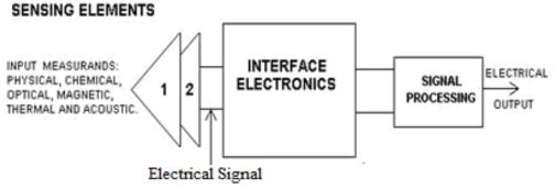
Fig.2 -Sensing elements and corresponding electrical signal
