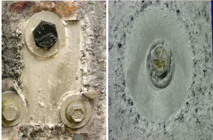
Fig. 4.2: (a) Corrosion testing of Magnesium casting alloy AE44 plate (b) Magnesium alloy AM60 plate, cold sprayed with aluminium
