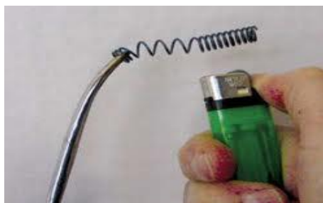
Fig no 1. A Deformed spring regaining shape on application of heat by a lighter
