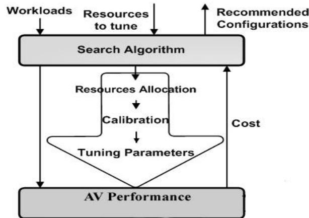
Fig. 8: The Automatic Cloud Antivirus Configurator (ACAC).
