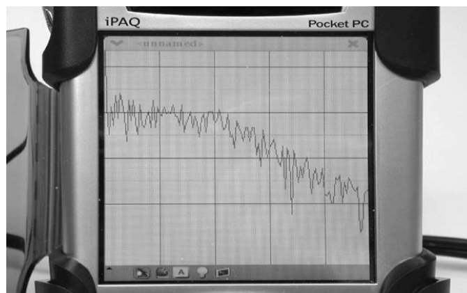
Fig. 4. Photograph of the front panel of the phonometer. Scales have been dropped to better exploit the limited display resolution. Scales range can be manually set by means of menus of a microphone. This application needs
