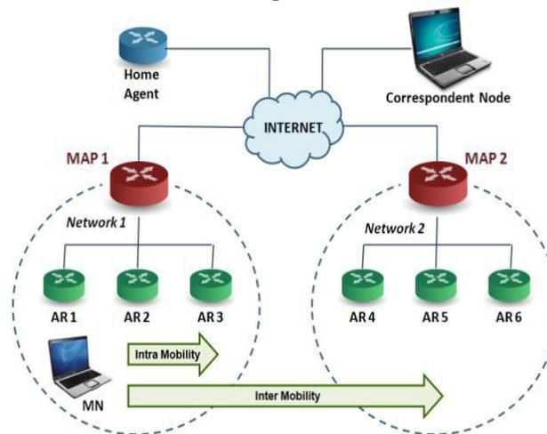
Fig2. Hierarchical Mobile IPv6 Architecture
