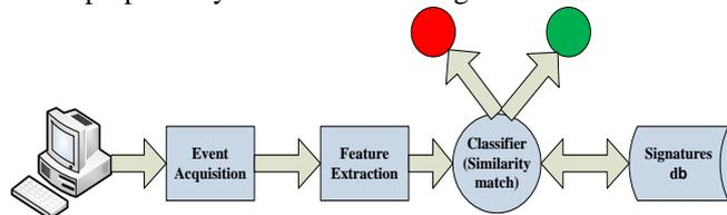
Fig.1 General Block diagram of proposed system
