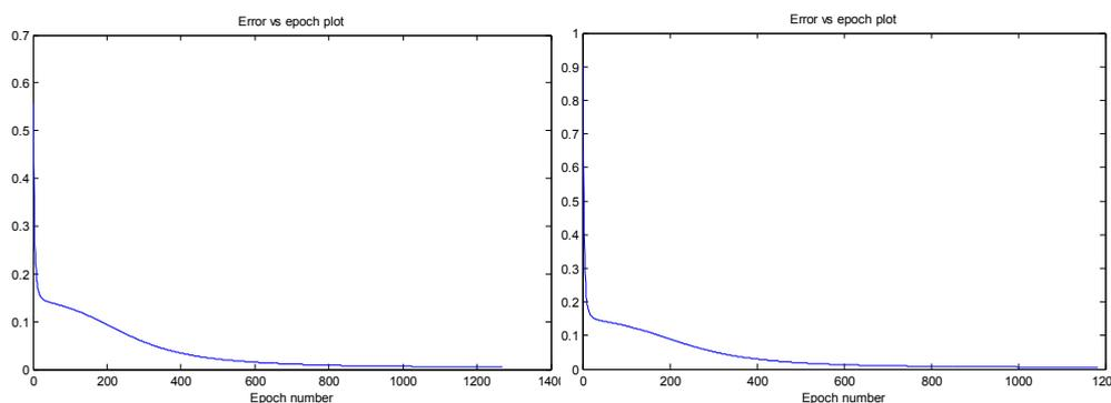
**Figure 2:** Two typical plots of the instantaneous squared error on an epoch by epoch basis as training proceeds
