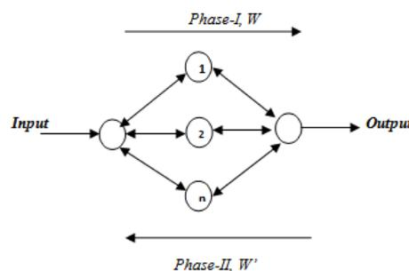
**Figure 1:** A typical 1-n-1 feed-forward architecture as Bidirectional Associative Memory
