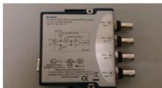
Figure 3: NI-9234 DAQ Board
