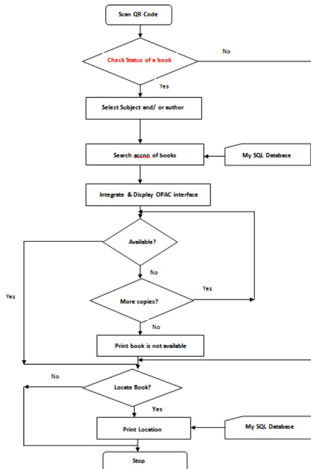
Fig.2 Control Flow Logic
