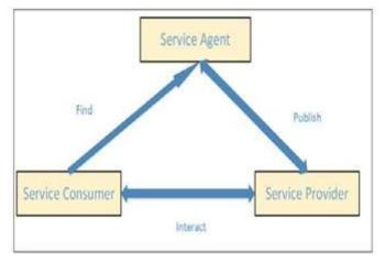
Figure 2: Service-Oriented Architecture model
