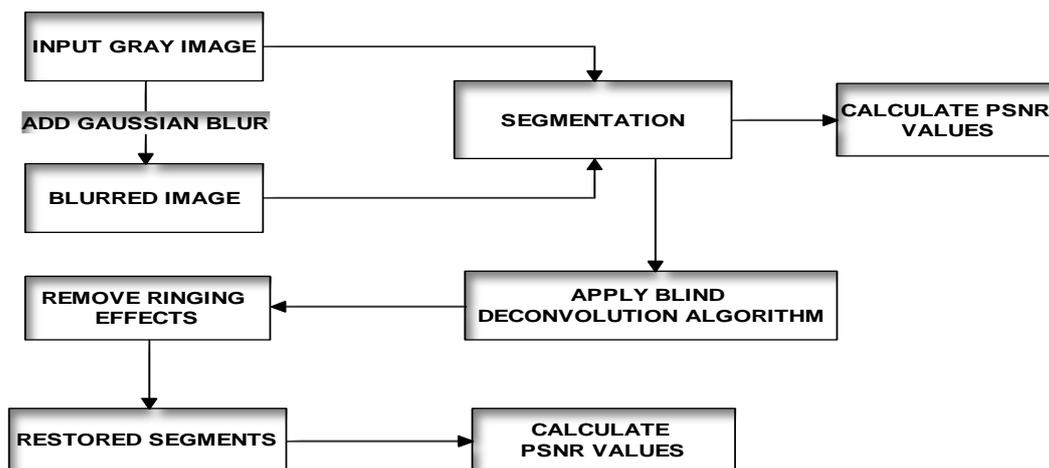
Fig (2): Architectural Model Of Proposed Technique.
