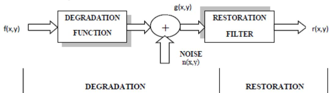
Fig (1): Degradation Model
