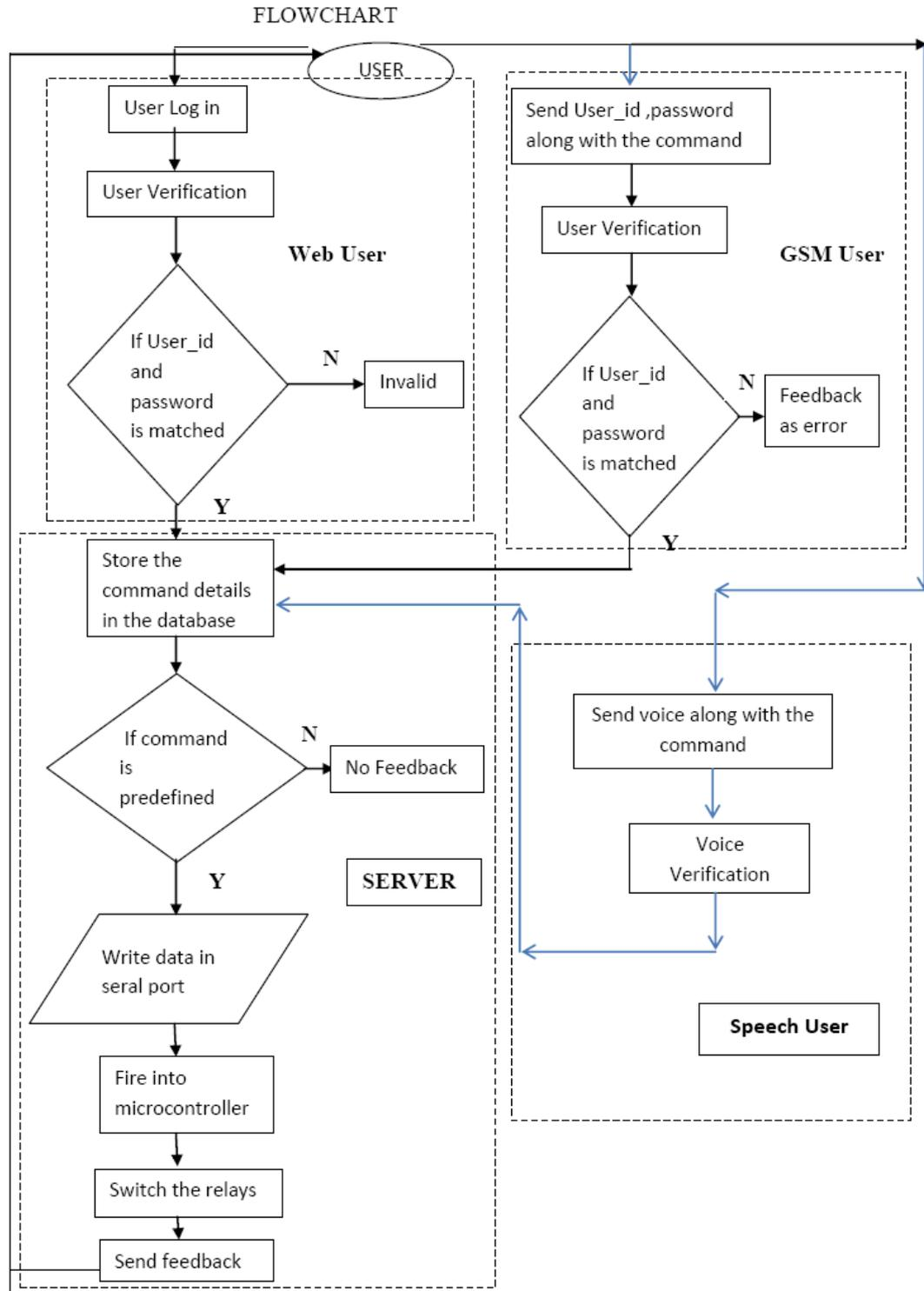
Figure 3.2 Proposed flow-diagram
