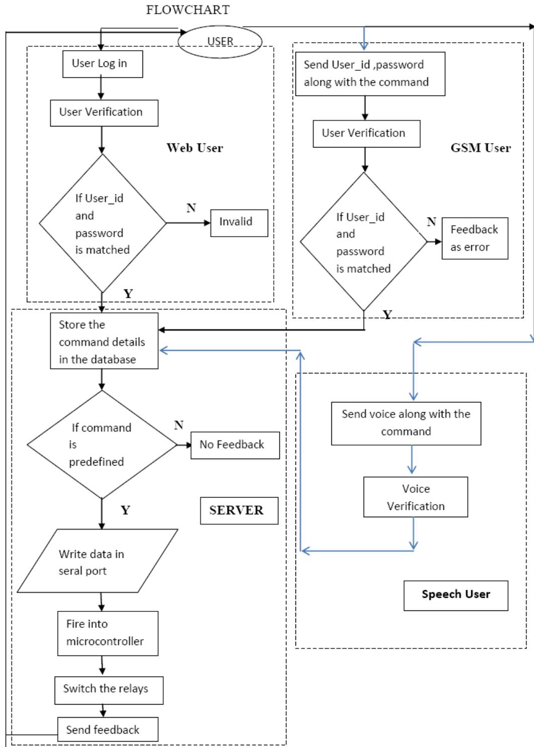
Figure 3.2 Proposed flow-diagram
