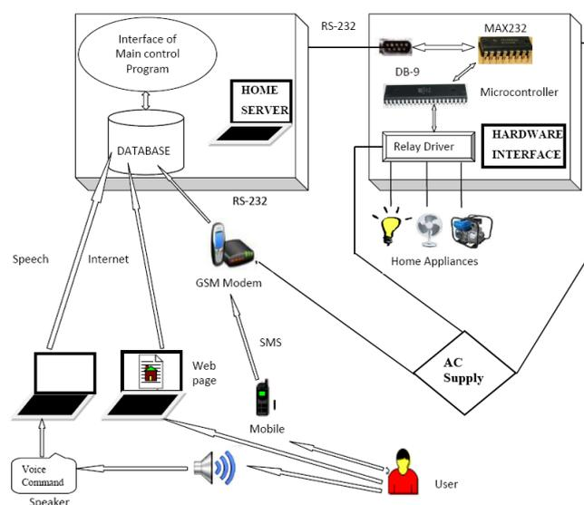
Figure 3.1: Block Diagram of overall proposed system
