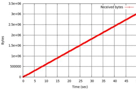
Fig.11. Total bytes received for UDP- interoperation
