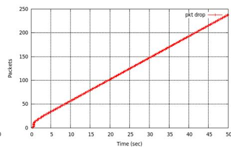
Fig.7. Total packets drops of UDP- interoperation
