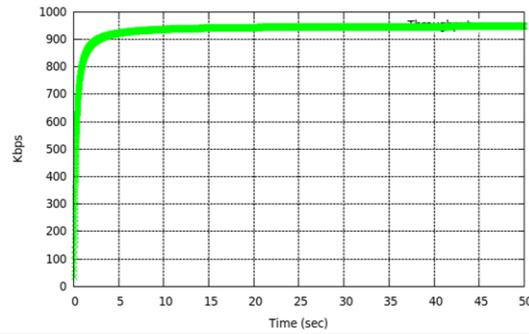
Fig.3. Instantaneous throughput of UDP- Interoperation
