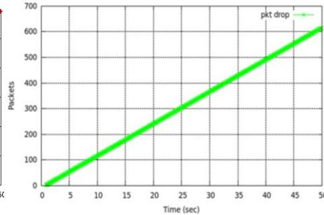
Fig.5. Total packets drop for UDP- independently
