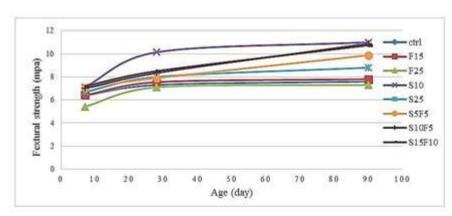
Figure 3. Flexural strength of concrete mixtures
