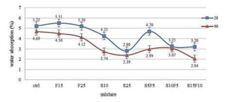
Figure 4. Water absorption of concrete mixtures
