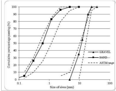
Figure 1. Particle size distributions of aggregate
