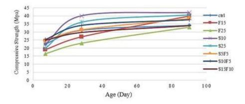
Figure 2. Compressive strength of concrete mixtures
