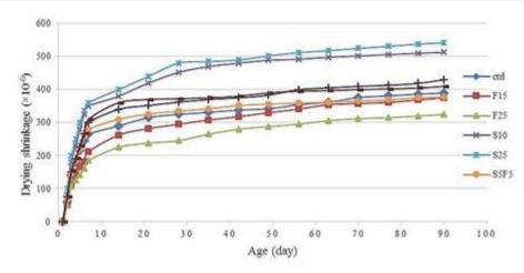
Figure 6. Drying shrinkage of concrete mixtures
