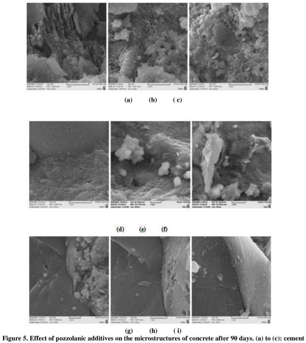
paste of Control sample, (d) to (f): cement paste of Silica fume (10%), (g): concrete sample of control, (h): concrete sample of F15, (i) concrete sample of S10
