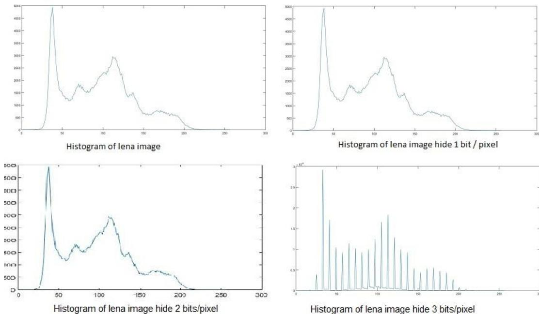
**Figure 4** Histogram of Lena image and after hiding 1,2 and 3 bits per pixel
