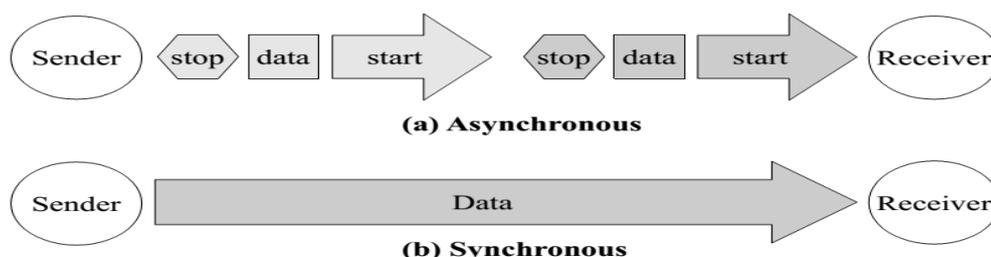
Figure 3: Types of message exchange. Synchronous and Asynchronous [6]
