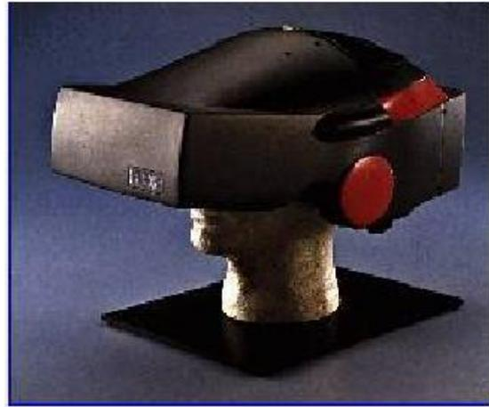
**Figure 2** A head mounted display (HMD)
