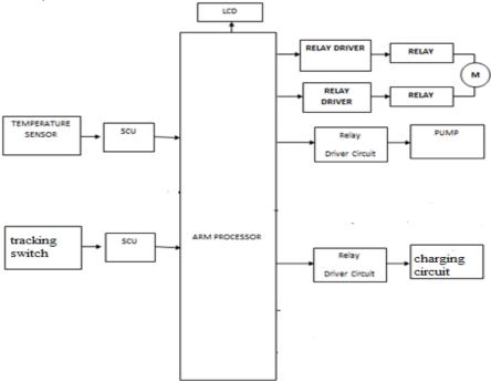
Fig 2.1 Blocks Diagram Of Proposed System
