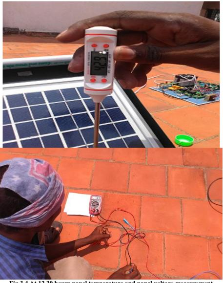
Fig 3.4 At 12.30 hours panel temperature and panel voltage measurement
