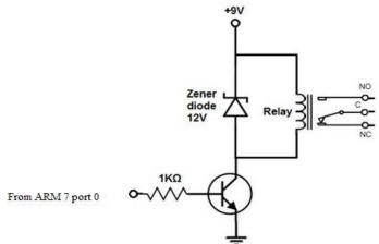
Fig 2.3 Relay Driver Circuit
