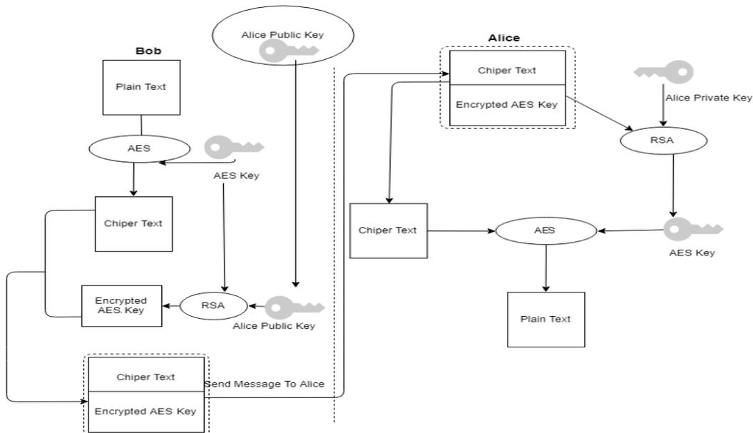
Fig.4.1 RSA 4096 Simple working process:-
