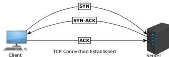
**Figure 2:** Normal TCP three-way handshake
