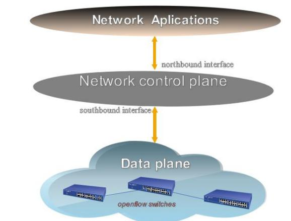
**Figure 1:** A simplified SDN architecture
