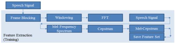
Figure 2 Block diagram of MFCC Feature extraction
