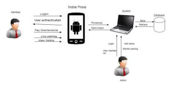
Fig6.1: System Architecture
