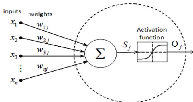
Figure 3: Artificial neural network active node<sup>25</sup>
