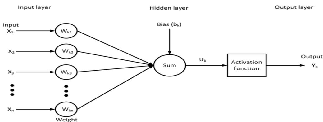
Figure 1: Standard Neural network structure
