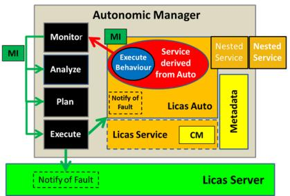
Figure 2. Schematic of the licas service architecture.
