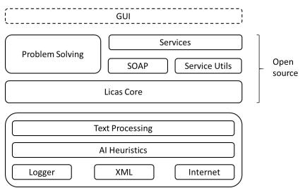
Figure 1. The licas software stack.
