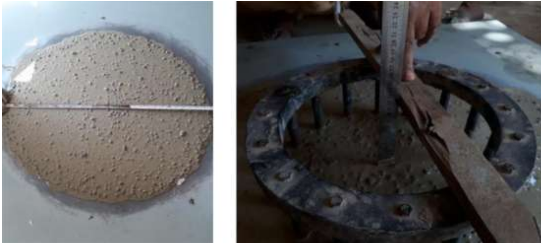
Figure 7. Pictorial views of slump flow and J-ring tests
