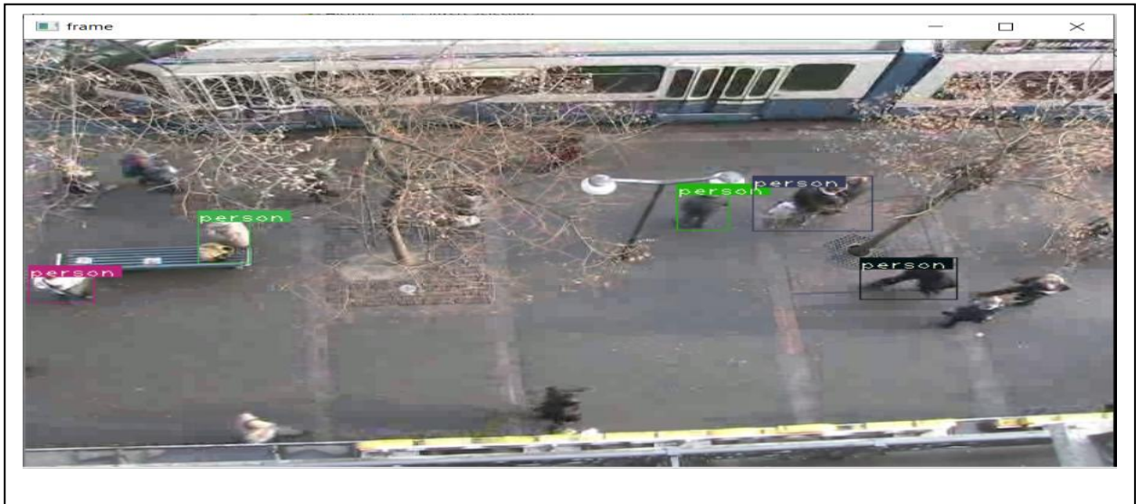
Figure(II) Pedestrian detection through surveillance system using YOLO v3 on ETH Dataset
