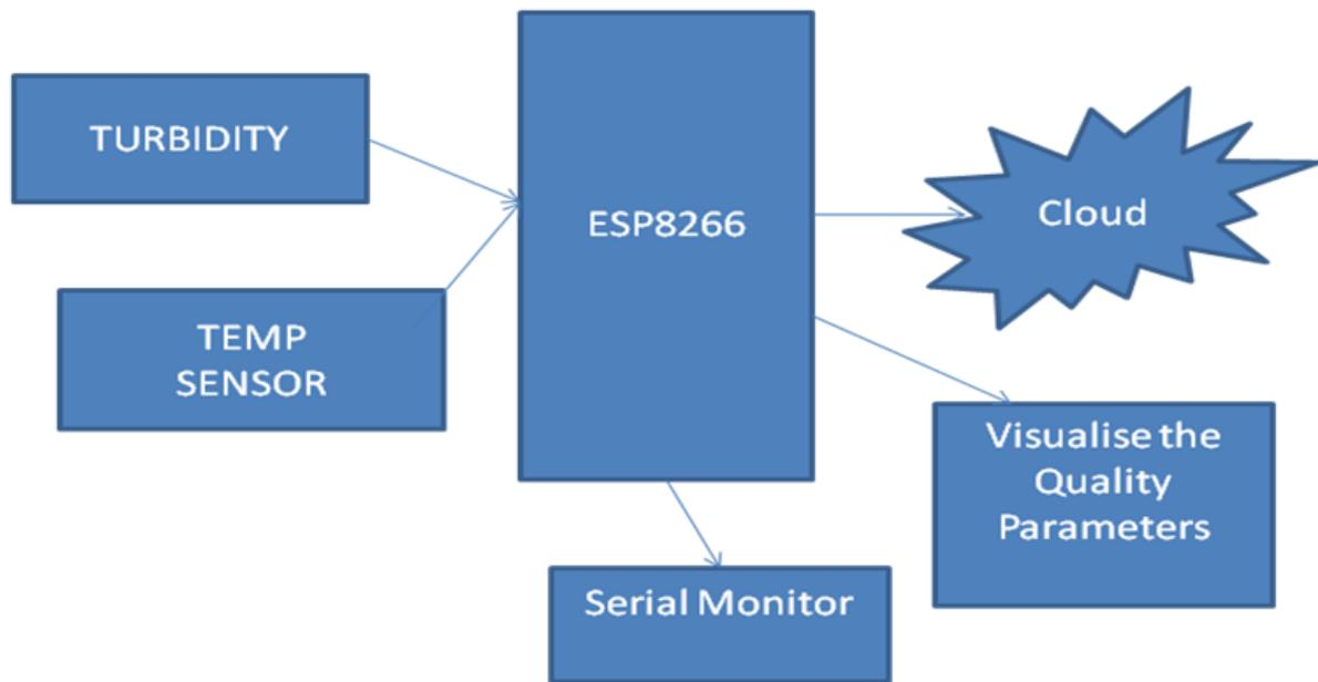
Fig. 1. Block Diagram of the Proposed System
