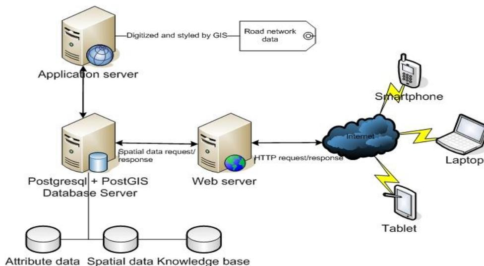
**Figure 1:** 4-tier Architecture of the Proposed GIS-system
