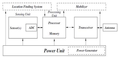
Figure 1:General hardware architecture of a sensor node.
