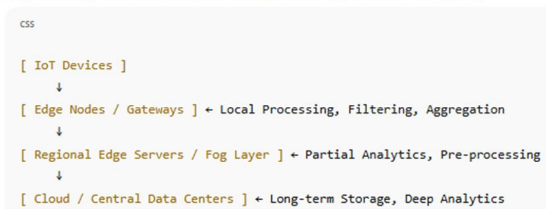
Figure 1: Edge-enabled IoT System Architecture (Illustrative Description)
