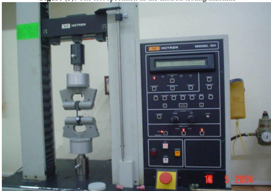
Figure (3): The test specimen in the Instron testing machine
