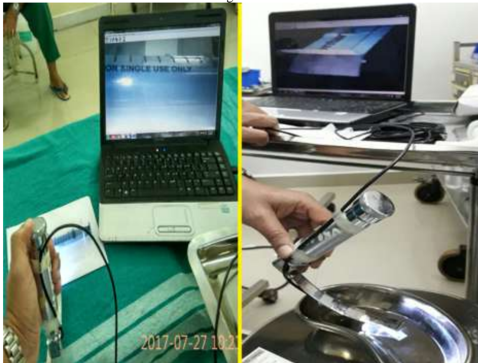
Checking for orientation of camera in first half of the figure and the second half it's dipped in water and it focuses on the sticker stuck to bottom. Its water proof, wash and reuse like Macintosh blade.
