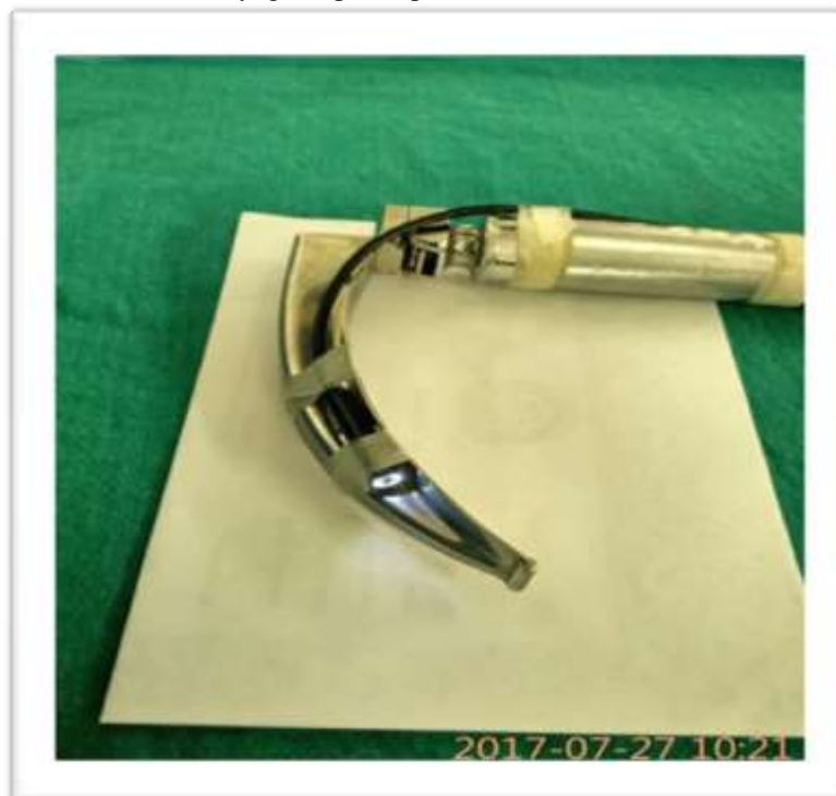
Figure: 7 Setting the video laryngoscope. LED lights whose intensity are adjustable .
