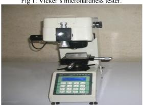
Fig 1: Vicker's microhardness tester.
