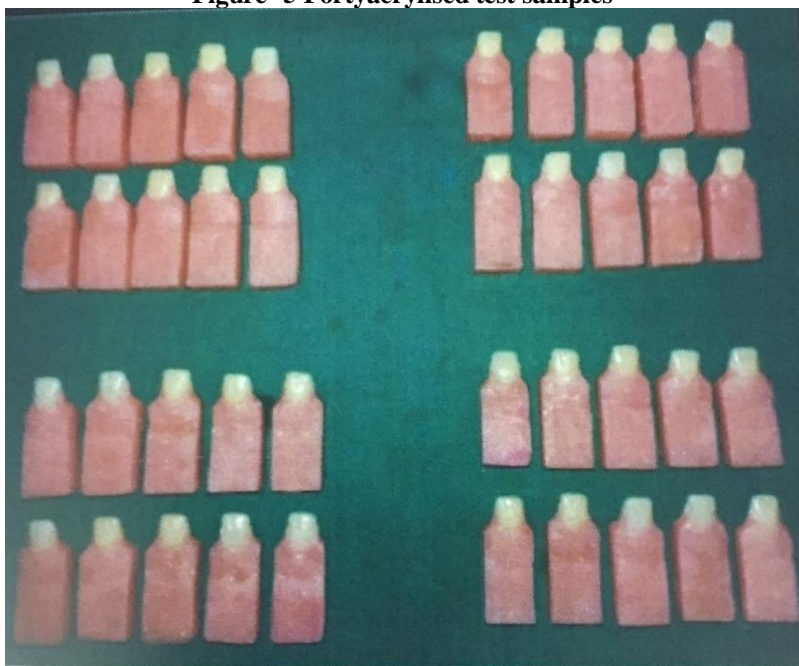
Figure- 5 Fortyacrylised test samples
