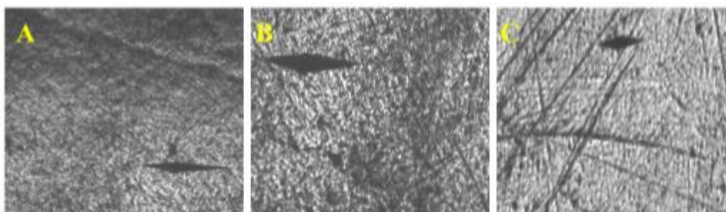
(Fig. 24): Images of knoopmicrohardness test indents of Samples remineralized by Pro Fluoride varnish(A), MI varnish(B), Icon(C)
