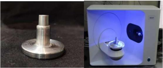
Fig1:Stainless SteelMasterDieFig2:Scanning ofmaster die with Medit T310 lab scanner
