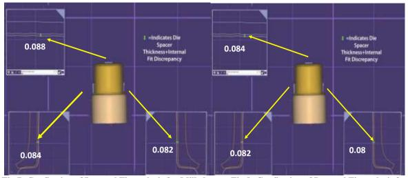
Fig 7: Cut Section of Internal Fit analysis for Milled Co Cr copings with 65 µm die spacer thickness
