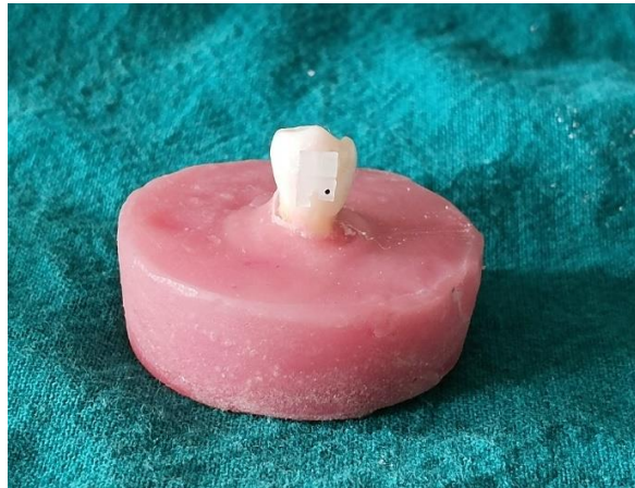
Figure 1. The prepared sample with bonded ceramic brackets
