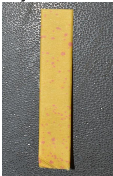
Figure no 5 – UIP turning red on contamination with citric acid solution
