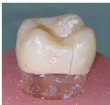
Figure (3): (Class I) crack started from point of load application propagates up to mesial surface until reach margin.
