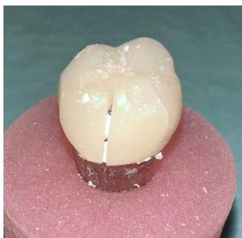
Figure (4): (Class II) with two fracture lines: one fracture line propagated from occlusal surface to palatal surface until reach the margin and the other propagated to mesio-palatal line angle.
