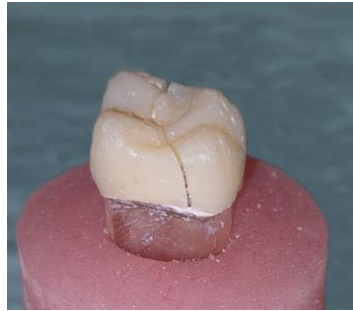
Figure (5): (Class III) fracture path propagated from occlusal surface in mesio-distal direction, results in splitting of the specimen into two equal parts.
