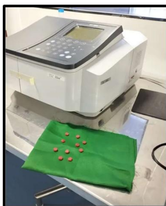
Figure 5: Specimens tested using colorimeter
